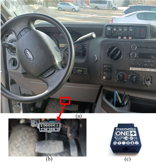
Fig.3 The minibus cabin showing the OBD port and OBD data logger for data collection
